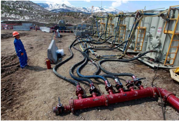
Use of water for hydraulic fracturing of gas-producing formations in Colorado's Piceance Basin.
